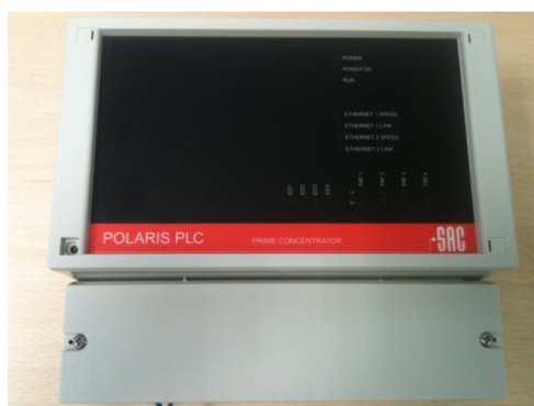
Figure 11 –Building Data Concentrator (BDC) prototype
