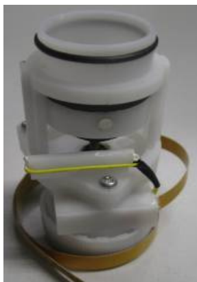
Figure 10 –Smart valve prototype
