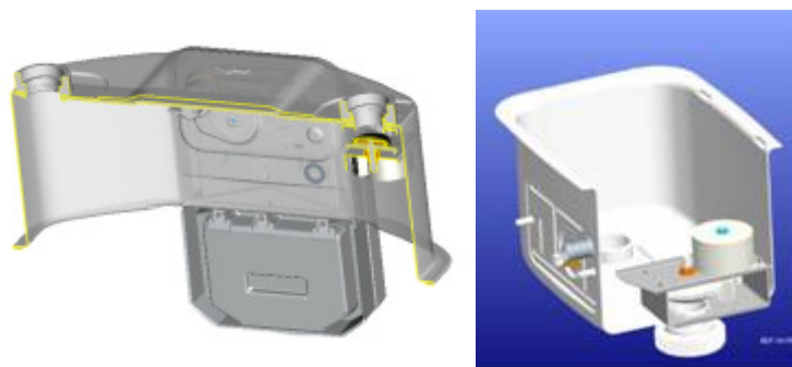
Figure 9 – Integration design of a valve driven by a stepper motor
