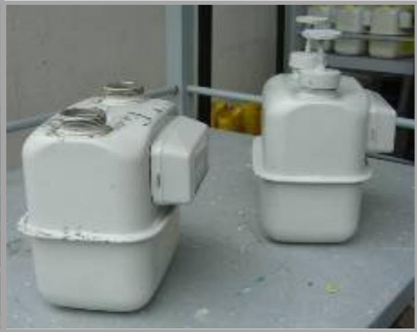
Figure 7. Photographs of meters before and after painting
