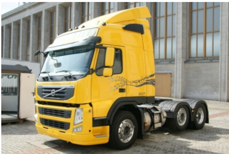
Figure 3: Volvo Dual Fuel (Natural Gas - Diesel) Heavy Duty Truck , Sweden
