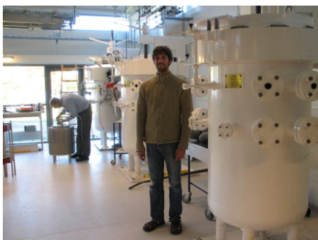
Figure 1. Photo of three autoclaves at Risø DTU for testing solid oxide cells up to 1000 \text{ }^\circ\text{C} and up to 10 \text{ MPa} (1 of them) and 5 \text{ MPa} .
