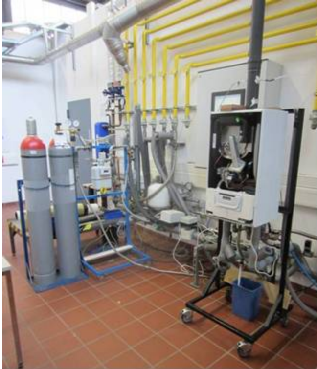
Fig. 9: Condensing boiler installed on the test stand in the lab at E.ON Ruhrgas in Altenessen
