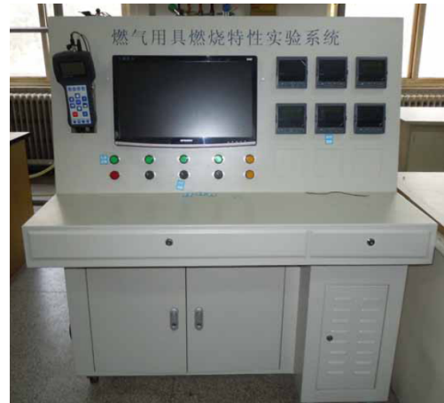
Fig. 16 Experimental test device of combustion characteristics of gas appliances used in CGAC
