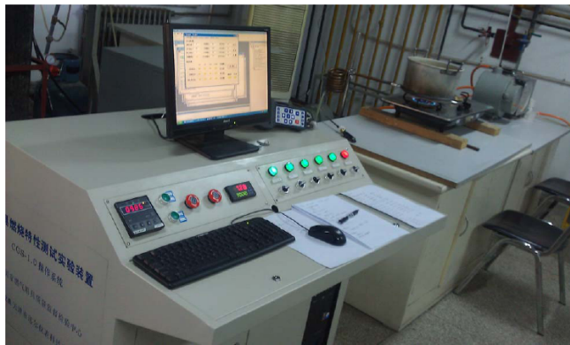
Fig. 16 Experimental test device of combustion characteristics of gas appliances used in CGAC
