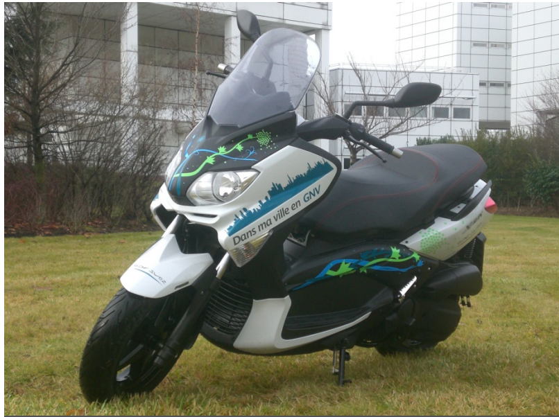
Figure 7: Prototype of scooter powered with CNG cartridges
