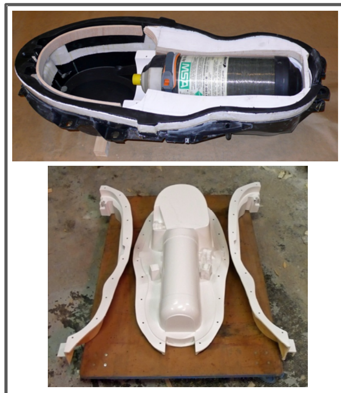
Figure 1 : Cartridge position into the cavity and moulds for the new cavity.
