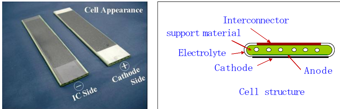
Figure 3. Appearance of the SOFC cell and a schematic drawing of the cross section
