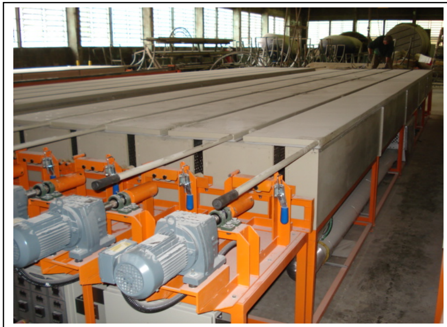
Figure 4: Curing and post-curing developed natural gas kilns – in operation
