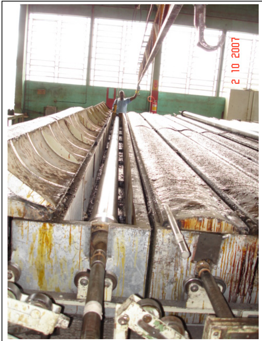
Figure 2: Electric kilns of curing and post-curing – mandrel placed
