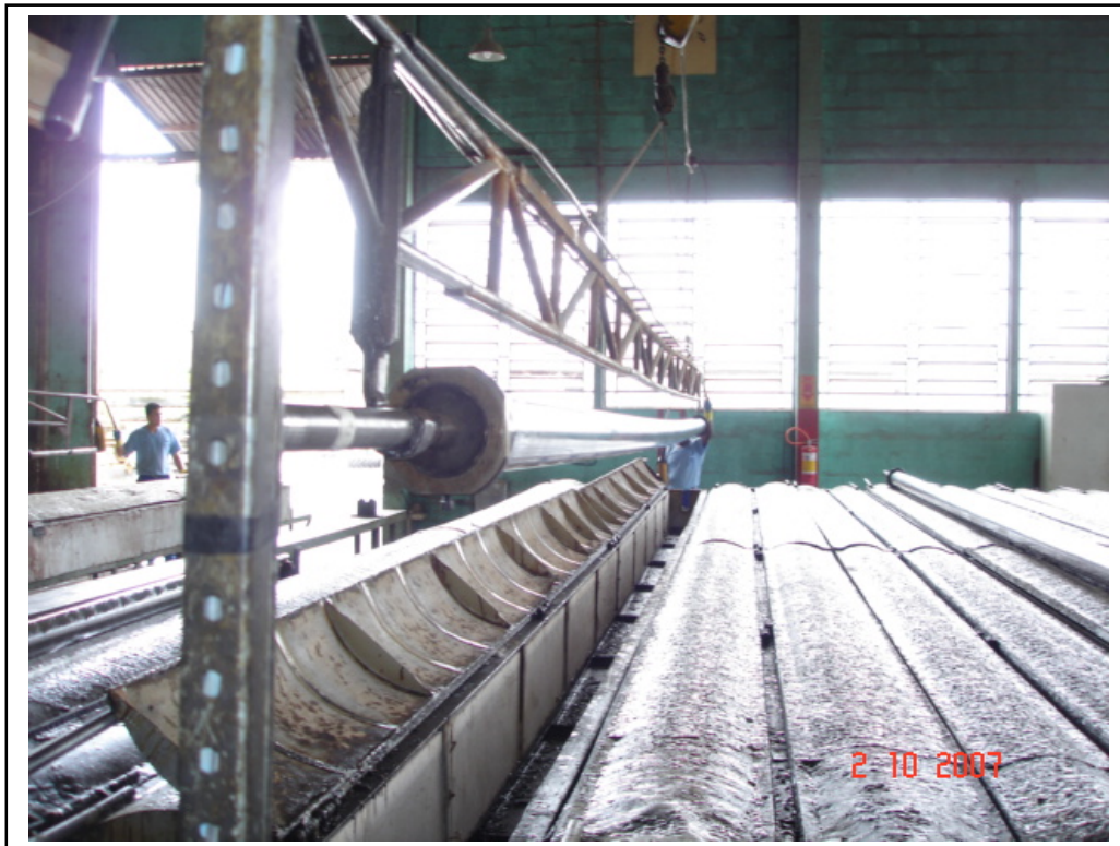
Figure 1: Electric kilns of curing and post-curing – material's loading
