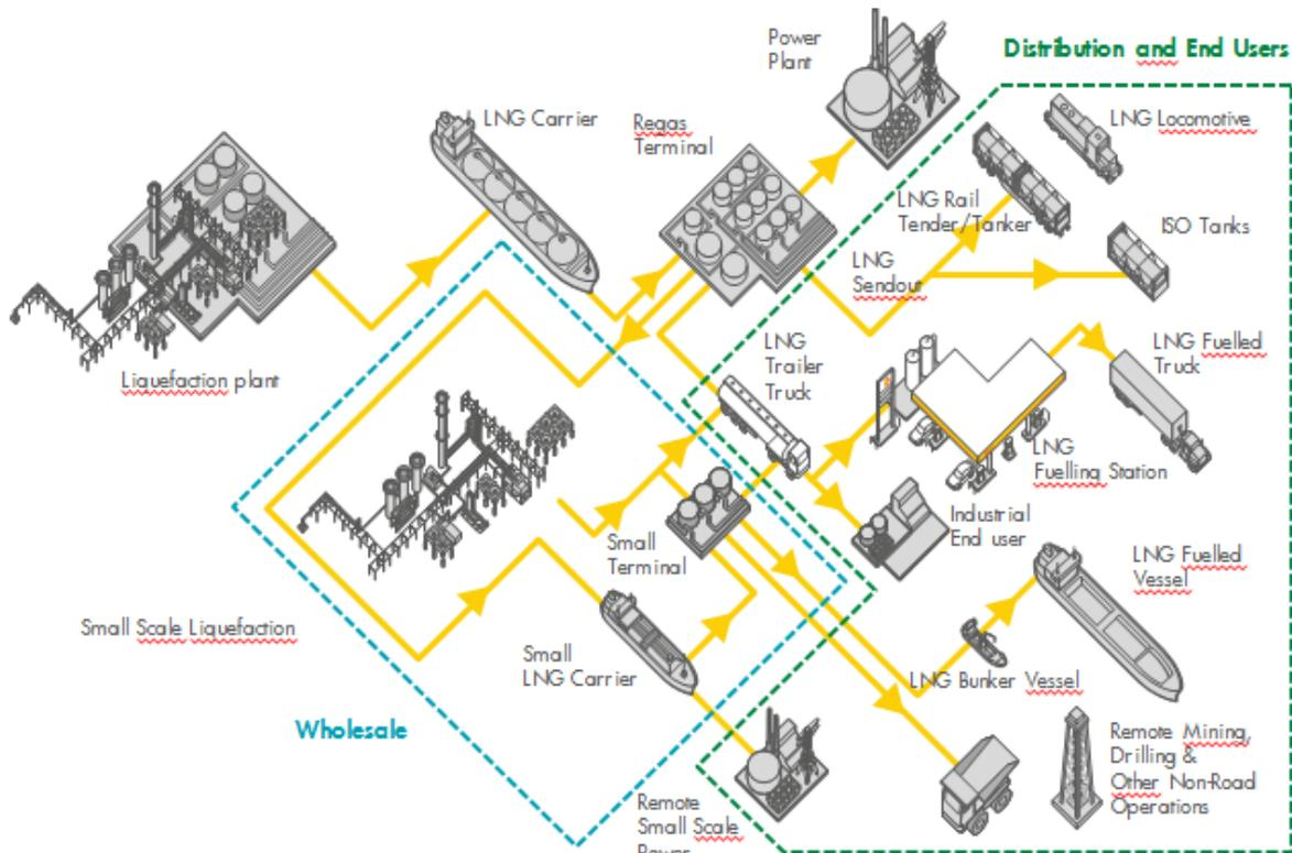
Figure 1 – Small-Scale LNG Value Chain
