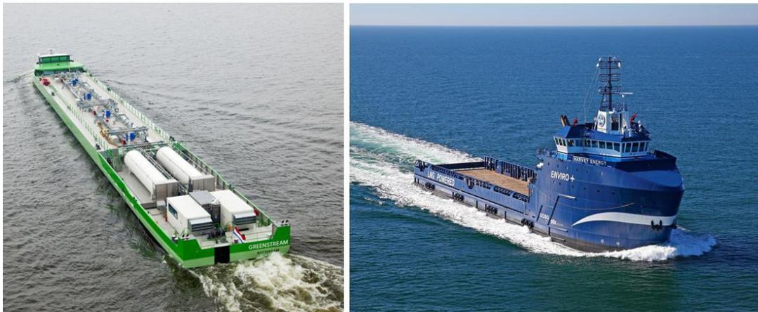
*Figure 7 – Developing LNG operating experience through LNG powered barges on the Rhine and Offshore Support Vessels in the Gulf of Mexico*
