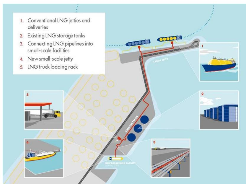
Figure 3 – Break Bulk at Gate Terminal, Rotterdam, Netherlands
