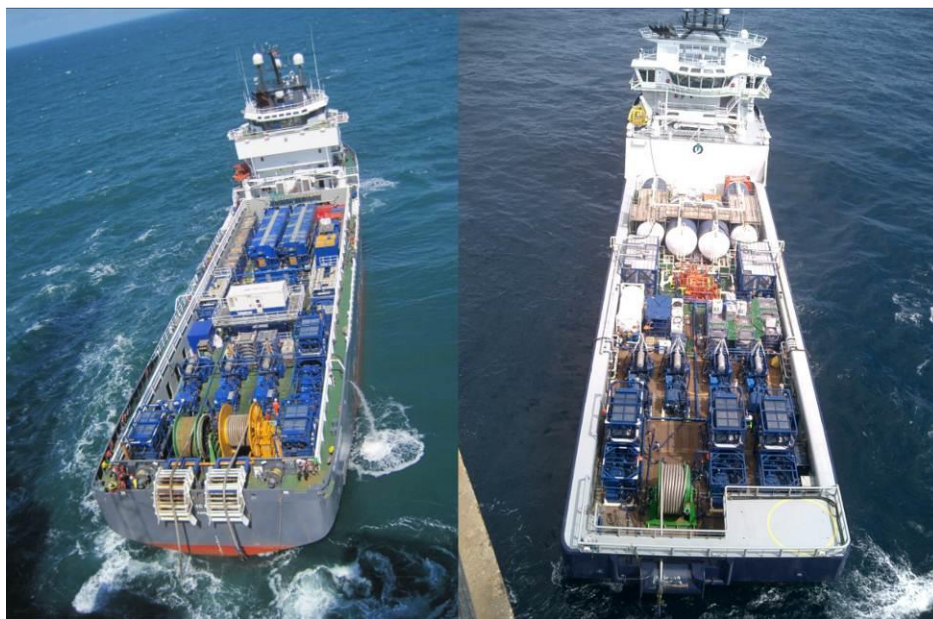
Figure 5: Two of the FlexSTIM vessels built in the North Sea during the last decade. Proppant fracturing set-up left and acid fracturing set-up on the right
