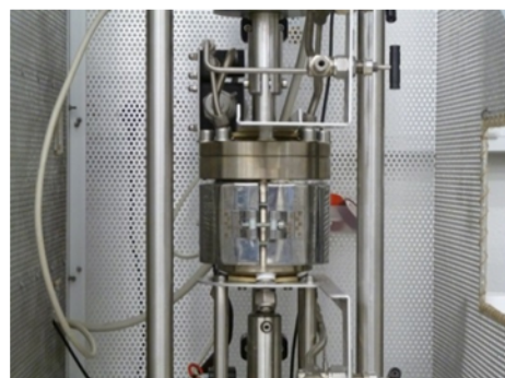
Figure 5: Testing tensile strength under hydrogen influence at Montanuniversität Leoben.
