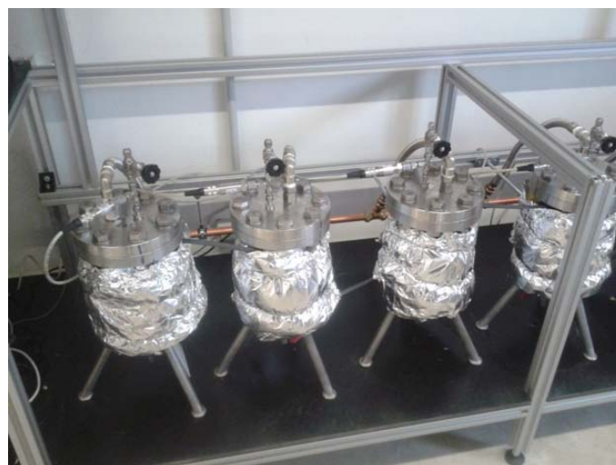
Figure 4: Bioreactors for testing microbiological activity under reservoir conditions at BOKU.
