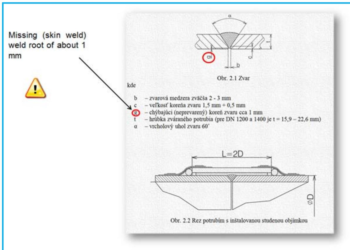
Fig. 3 Anomalous weld specification
