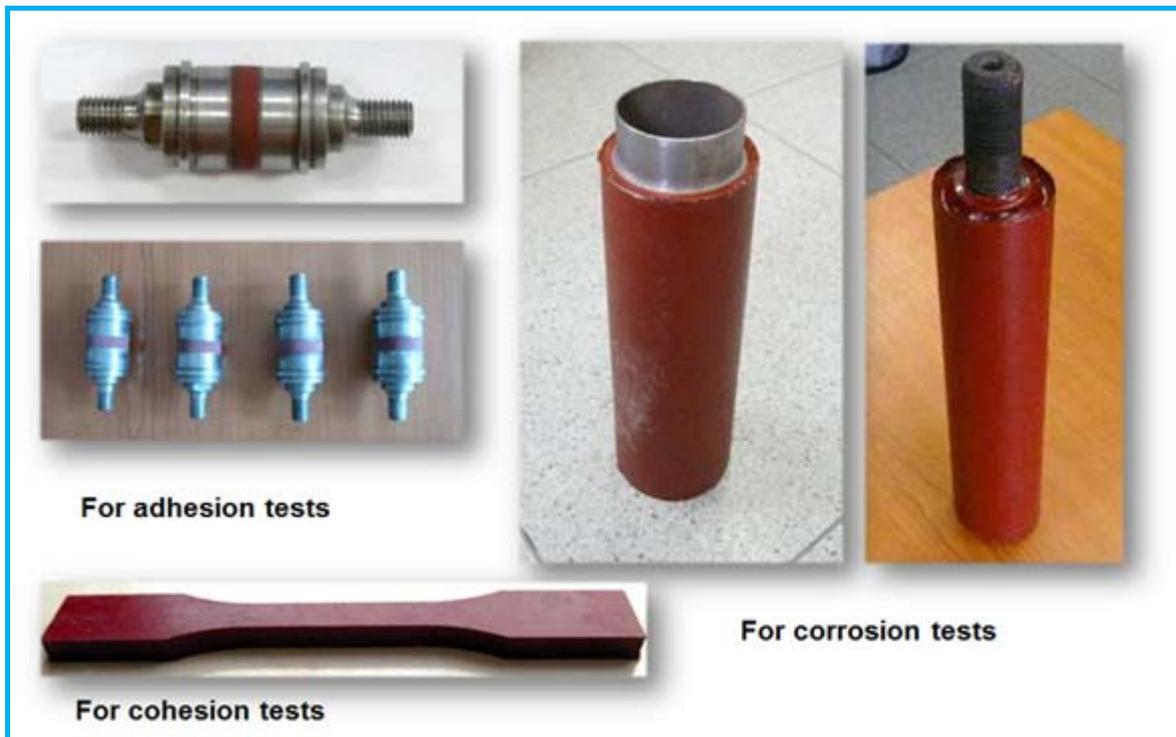
Fig. 4 Testing samples for mechanical and corrosion tests
