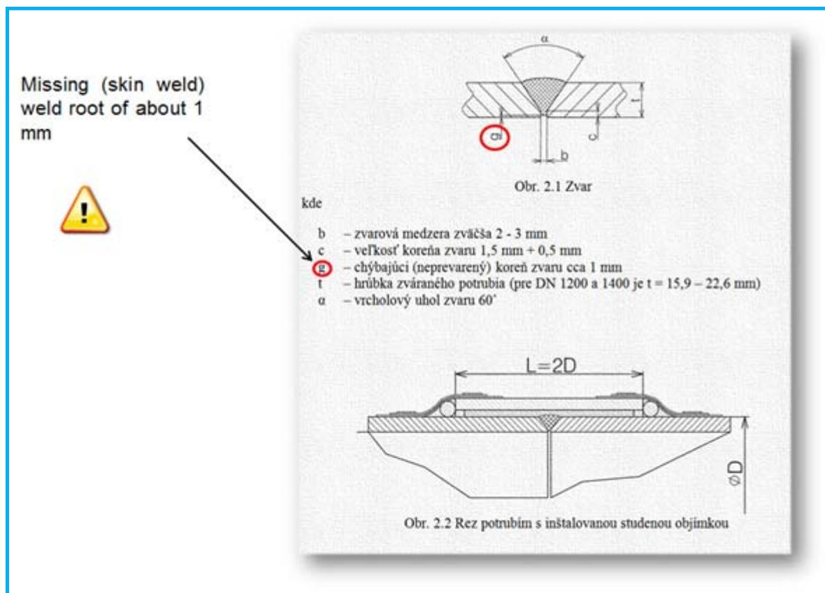
Fig. 3 Anomalous weld specification
