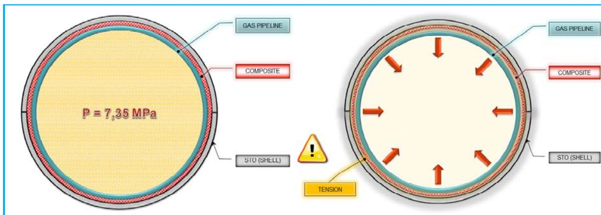
Fig. 2 Effect of the pipe depressurizing
