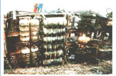
Remains of the natural gas bus. All cylinders are intact; no explosions occurred
