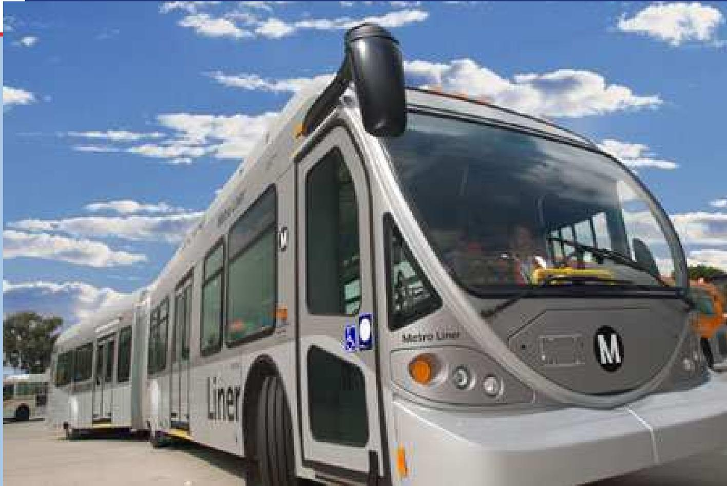
Los Angeles Metropolitan Transportation Authority's CNG-fueled "Metro Liner" buses are powered by the low-emissions Cummins Westport 320-hp L-Gas Plus engine.
