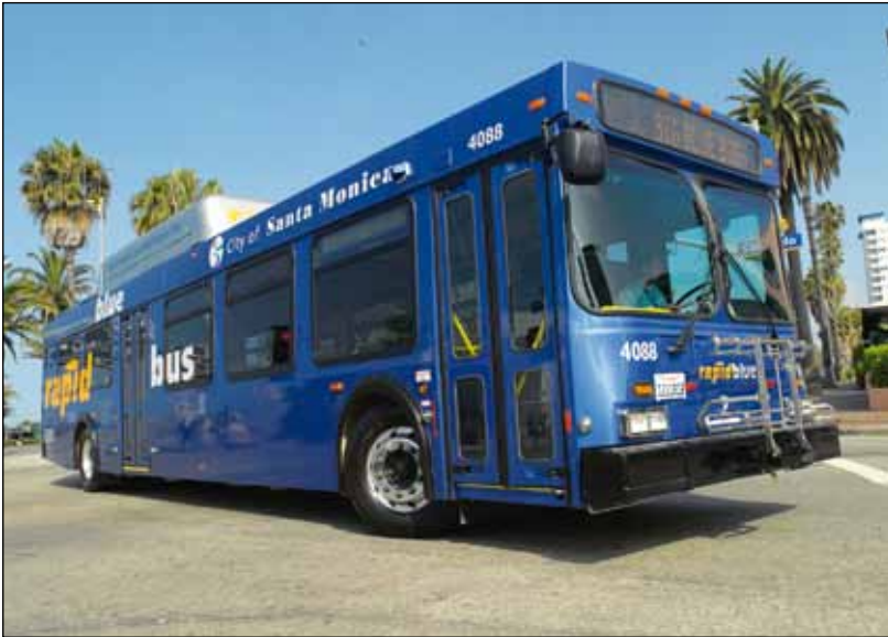
▲ US bus operators were early adopters of LNG fuel. Santa Monica's Big Blue Bus Line operates a fleet of more than 200 LNG (pictured), CNG and electric/gas hybrid buses in the Los Angeles metropolitan area.
