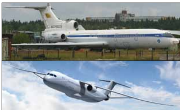
The Tu-155 has been retired (TOP) but Boeing has a concept for an LNG-fuelled airliner (ABOVE).
