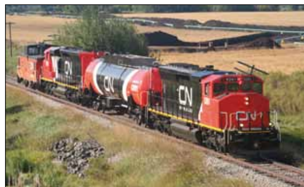
Canadian National Railway is trialling a dual-fuel LNG diesel set (two locomotives with a tender in-between).
