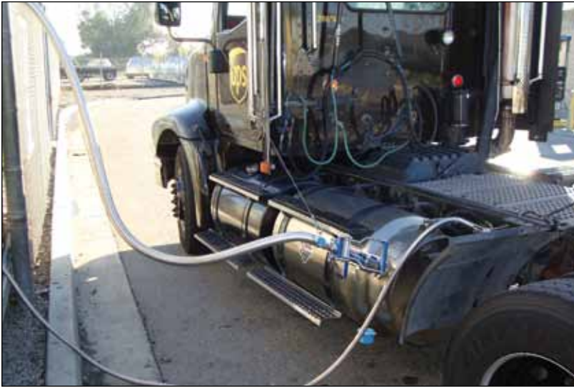
▲ UPS is using LNG to fuel its long-distance line hauling fleet in the US South-west.
