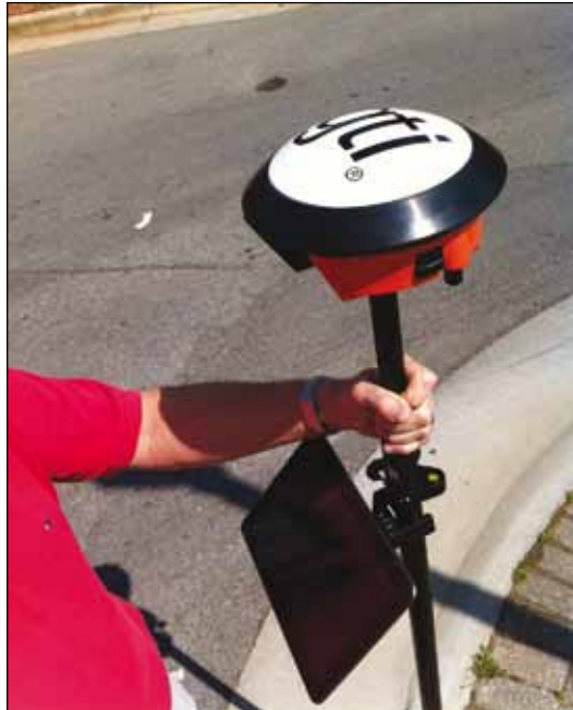
▶ Sub-metre accurate GPS providing data to a tablet computer running GIS-enabled software.
