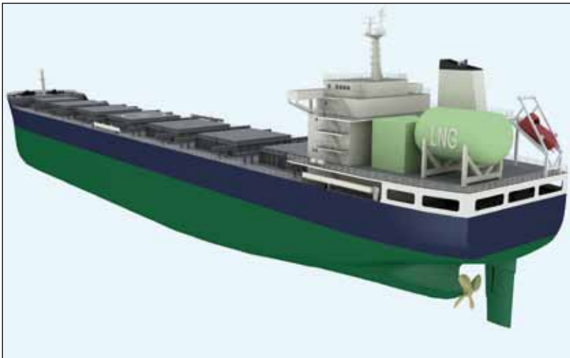
▲ The Clean Sky bulk carrier design has a single LNG tank on the port side.
