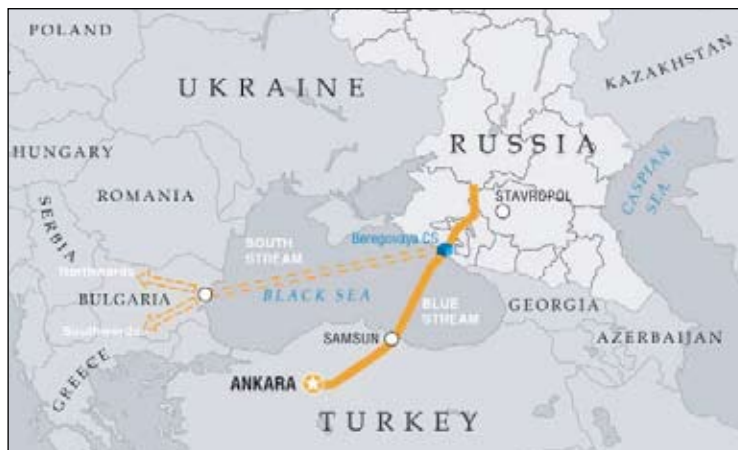
Blue Stream should reach its full design capacity of 16 bcm/year in 2010. The proposed South Stream pipeline would start at Beregovaya and make landfall at Varna before dividing into two branches.
