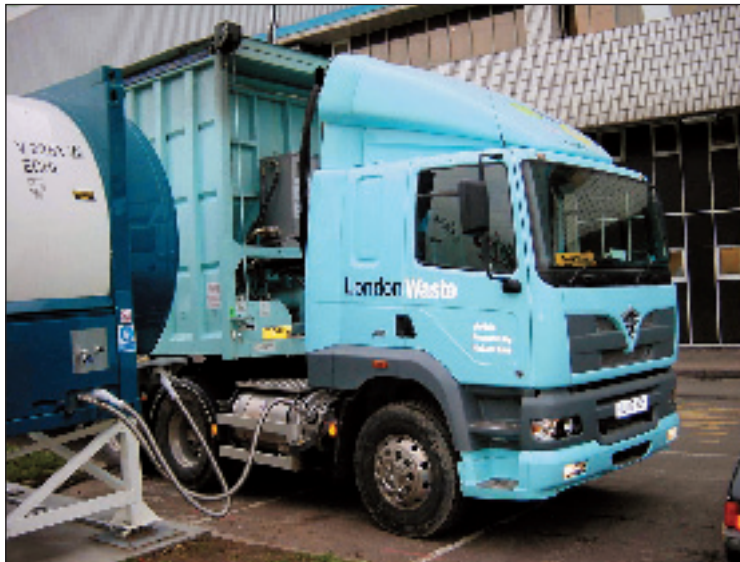
NGVs running on LNG tend to be larger, industrial vehicles such as this refuse truck in service in London.
