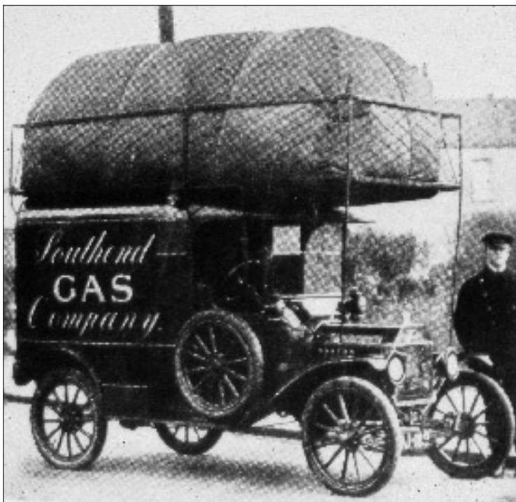
Early trials with gas-fuelled vehicles used uncompressed manufactured gas like this van operated by the UK's Southend Gas Company in 1934.
