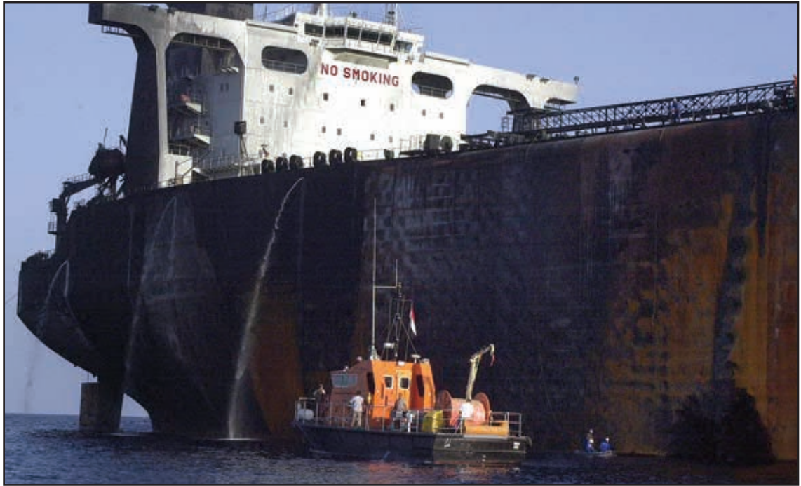
Although the Limburg 's cargo ignited when the ship was attacked it did not explode and the internal tank structure by the hole was undamaged.
