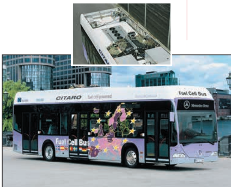
Ten European cities (Madrid is pictured) are involved in a trial of buses using PEM fuel cells. (INSET) The fuel cell unit with a power output of more than 200 kW and the pressurised cylinders containing hydrogen compressed to 350 bar are accommodated on the roof of the bus.
