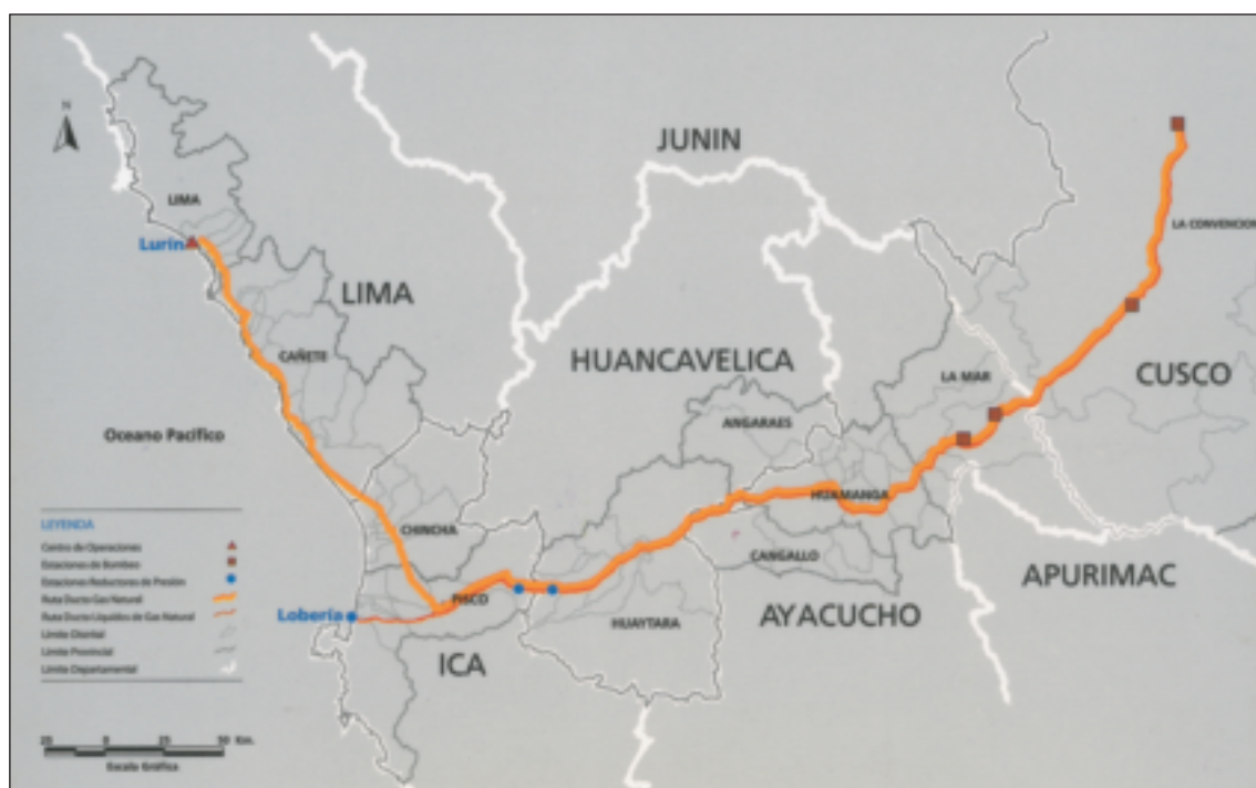
The map shows the pipelines transporting Camisea production of natural gas (orange) and natural gas liquids (red), whose construction faced major technical and environmental challenges with a rise in height to 4860 metres to cross the Andes before descending to the coast. A third pipeline will branch off and supply the Peru LNG plant which is being built in the district of Cañete.
