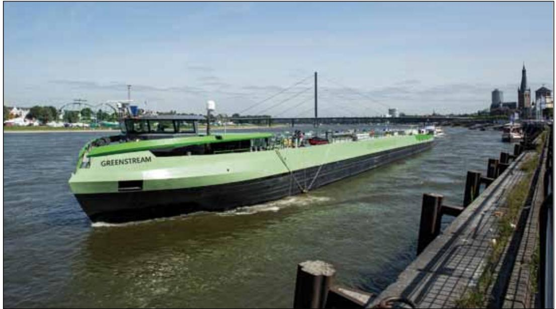
► The LNG-fuelled barge Greenstream started operations on the River Rhine in 2013.
