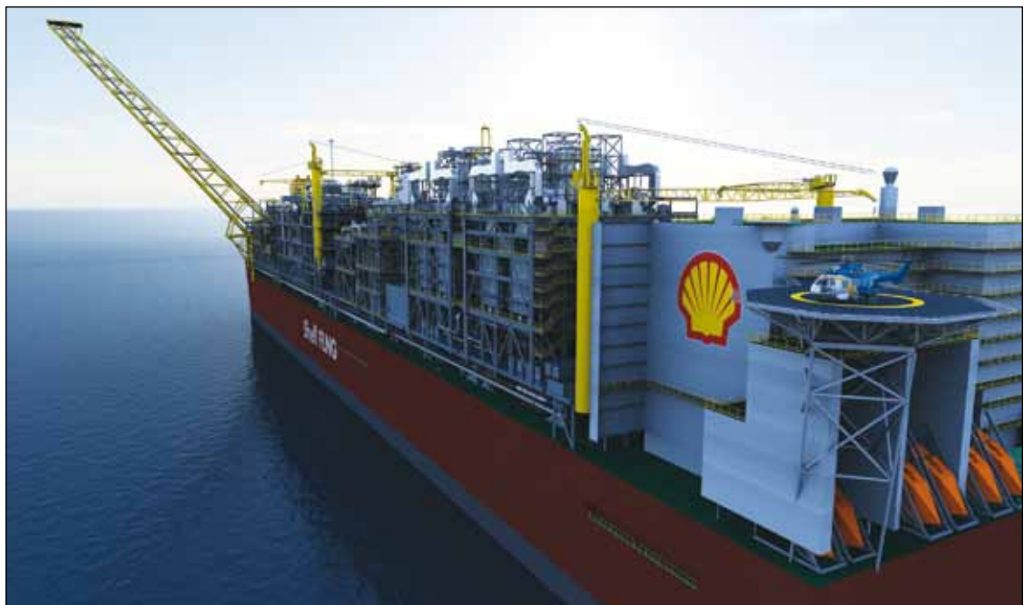
Prelude LNG's plant will be the world's largest floating facility with a displacement of 600,000 tonnes. It will be built by the Technip Samsung Consortium at Samsung Heavy Industries' shipyard in Korea.
