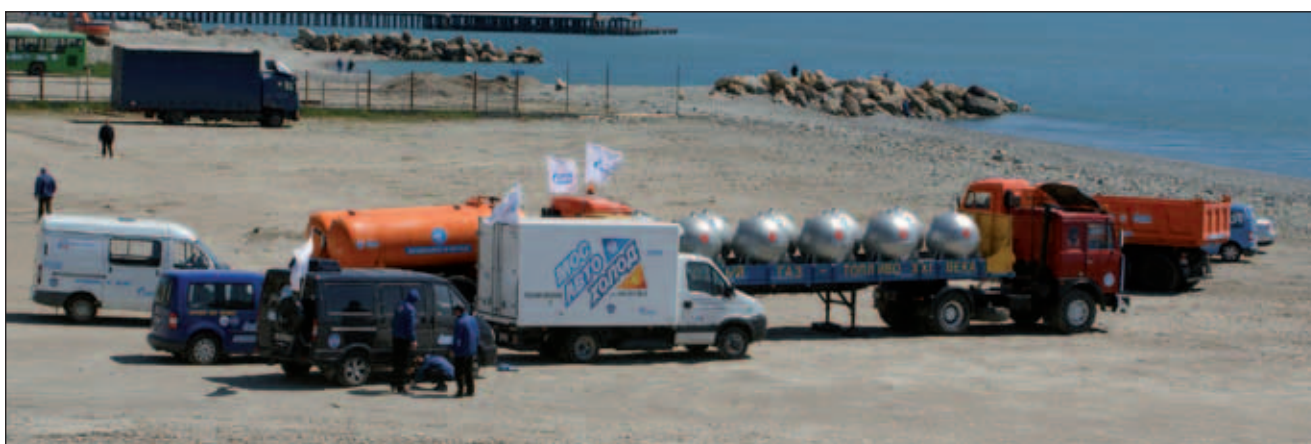
In addition to stops at permanent CNG filling stations some refuelling was done from a mobile CNG cascade carrier – in this case at Dzhubga on the Black Sea.
