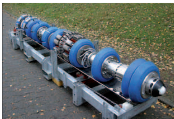
Figure 1: The new RoCorr·UT tool consists of an MFL and a UT unit and is available in sizes ranging from 6 to 40”.
