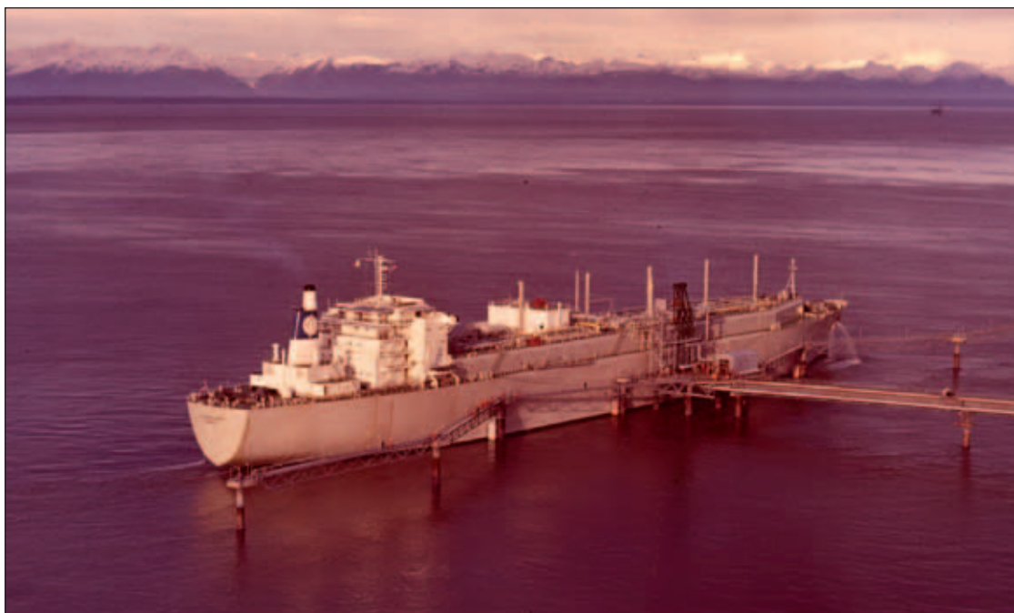
Asia-Pacific's first LNG cargo was delivered by the 71,500 m 3 Polar Alaska , which operated a shuttle service between Kenai and Yokohama with its sister ship Arctic Tokyo .
