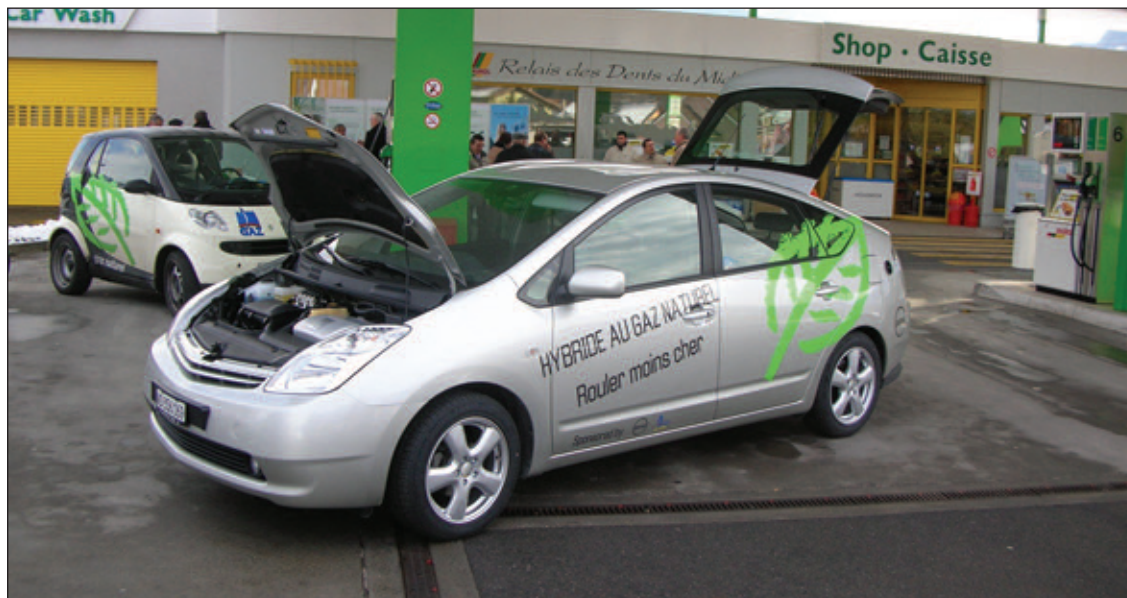
On display at the public refuelling station in Collombey are a Toyota Prius and Smart (background), both retrofitted by Holdigaz with a natural gas fuel system. (The Prius was also exhibited at the 23rd WGC in Amsterdam.)
