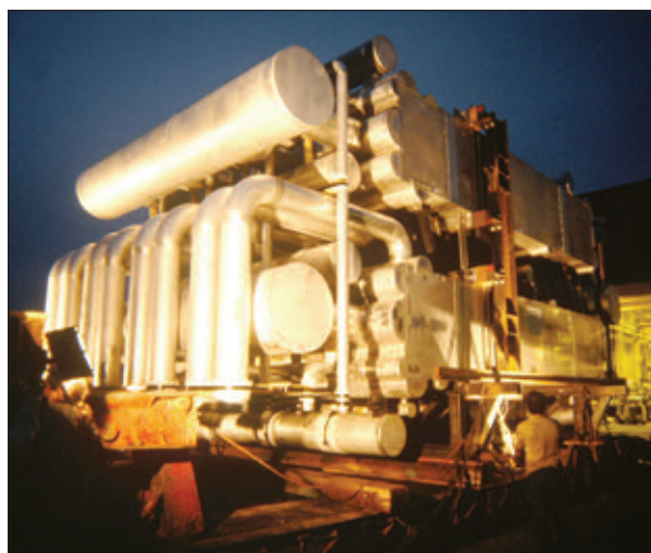
Chart's brazed aluminium heat exchanger core.
