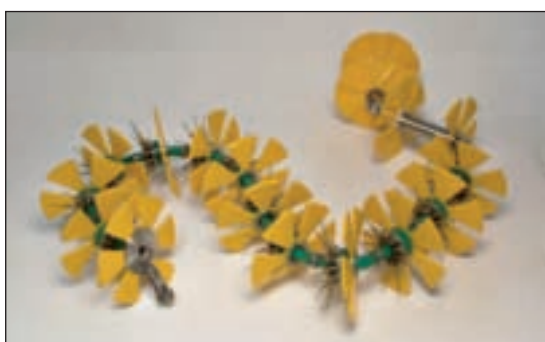
The feeler-snake pig: (ABOVE) a general view of electronics and sensor modules; (RIGHT) the pig being received from an offshore pipeline.
