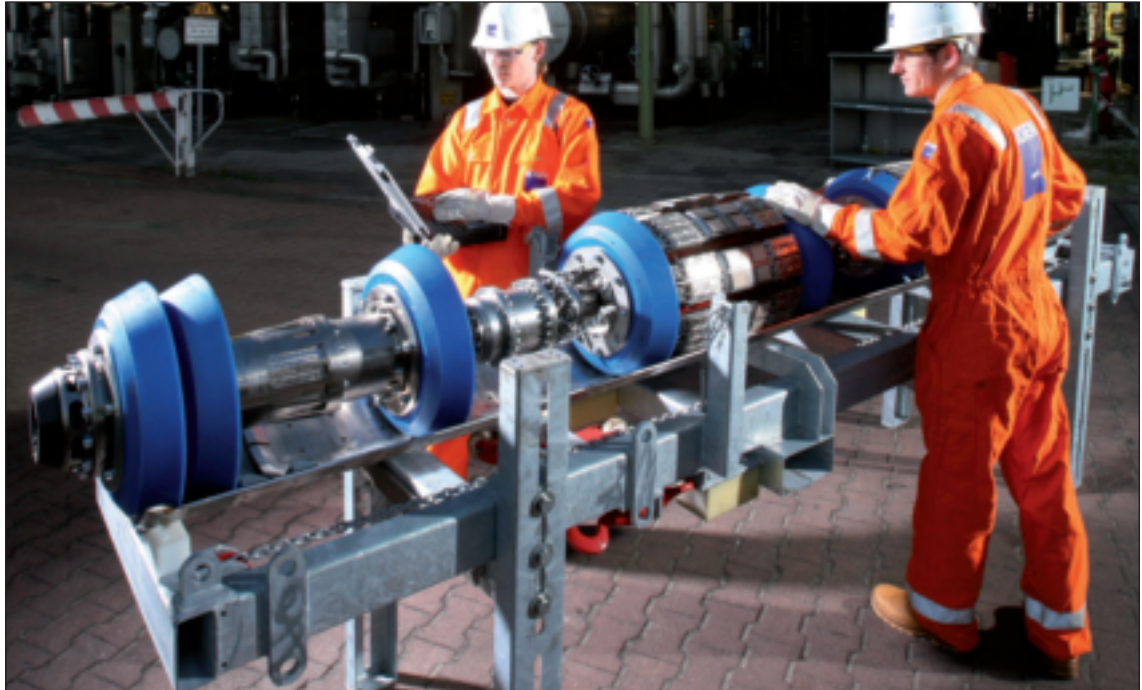
The new 16-in diameter inspection tool from Rosen Engineering designed for crack and coating disbondment detection.
