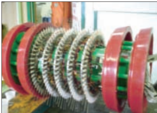
A 22-in diameter feeler pig with 250 sensors.
