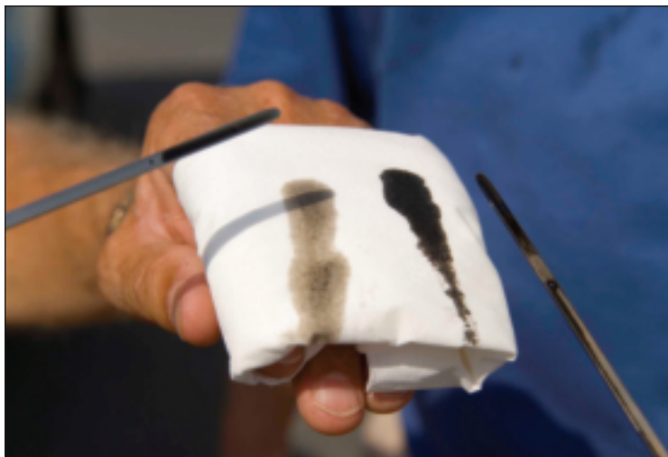
A simple dip stick test shows how much cleaner the GTL-fuelled vehicle (left) ran for over 10,000 kilometres compared to a 4500-kilometre sector with a conventionally-fuelled vehicle (right).
