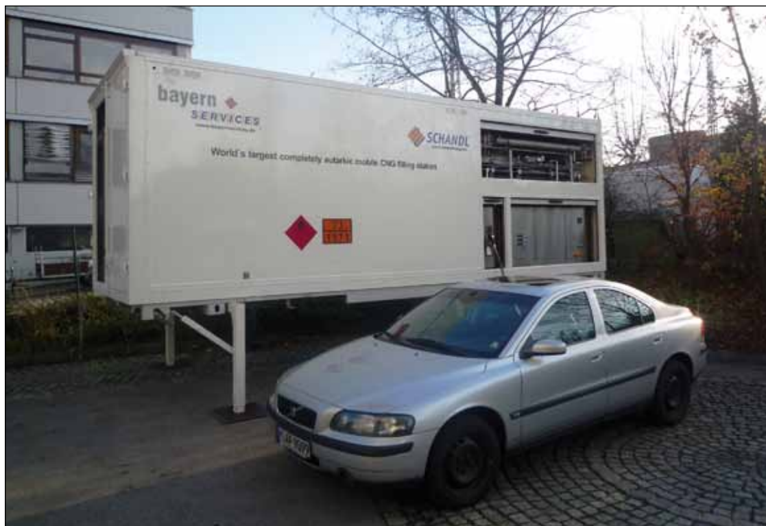
This mobile CNG filling station was inspected during the technical visit.
