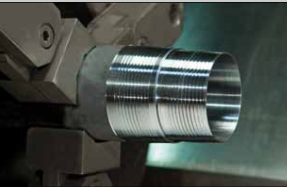
▲ Ultra Premium Connection threading at the Odessa Ultra facility.
