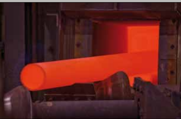
▲ Pipes undergoing heat treatment at TMK's Baytown facility.
