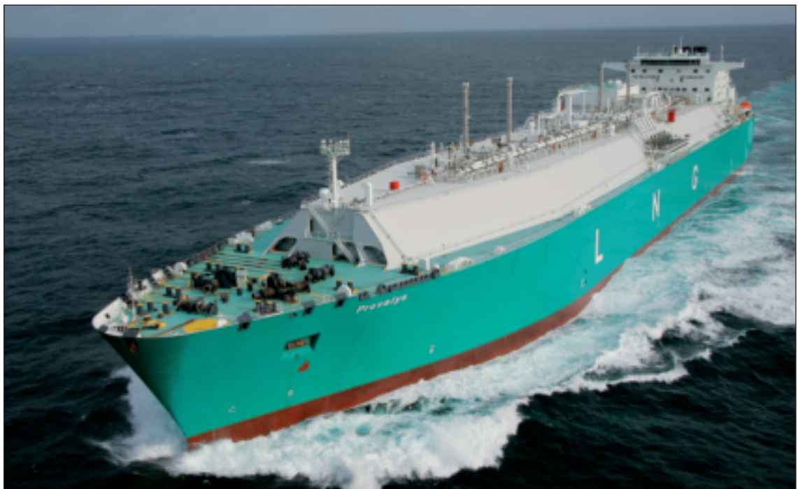
The 154,500 m 3 Provalys , the first LNG ship with a dual-fuel diesel electric propulsion system, entered service in late 2006.
