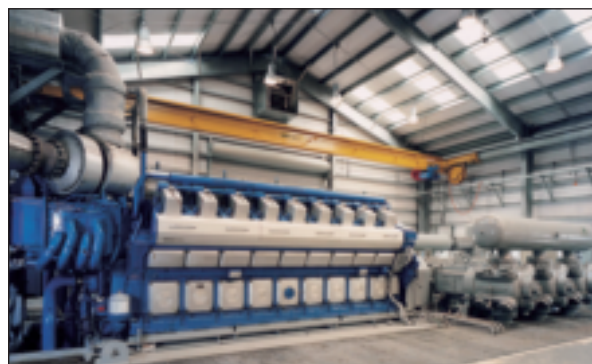
A Wärtsilä 34SG gas engine driving a 6 cylinder reciprocating compressor in an underground gas storage in the USA.
