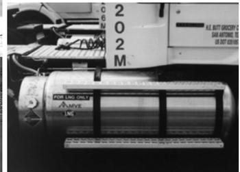
Fig. 9. LNG fuel tank
