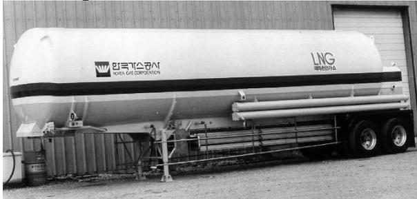
Fig. 3. LNG road semitrailer
