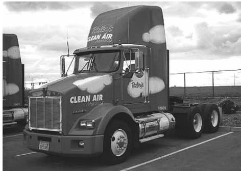
Fig. 8. LNG driven truck
