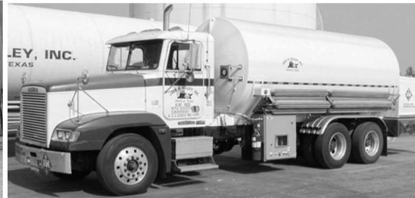
Fig 4. LNG delivery unit
