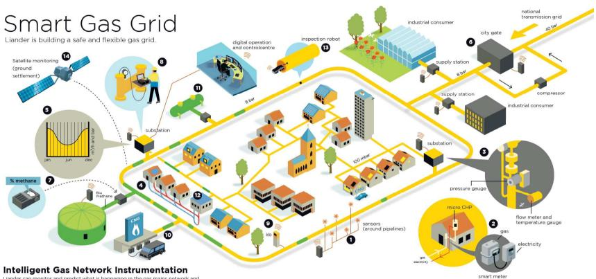
Liander can monitor and predict what is happening in the gas mains network and intervene in timegrid using remote measuring and control equipment.
